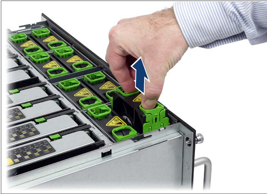
Figure 17: Unlocking a fan module and removing it
